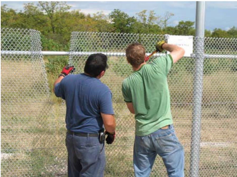
***Low threat consists of two men using hand tools to penetrate the barrier.***
