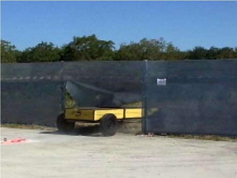
***The test vehicle totally penetrated an expanded metal panel fence system.***
