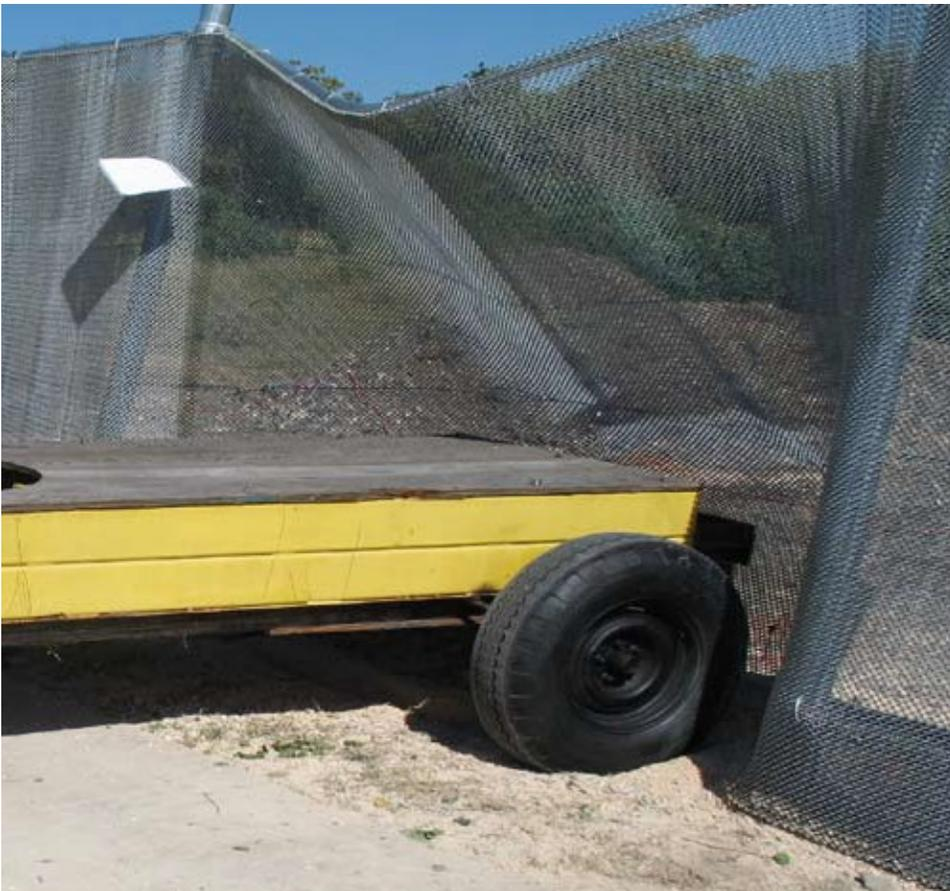
*Engineers designing safety and security systems for parks and other public works projects can use this research information to specify the correct security grade chain link fence system to meet these vehicle impact safety standards and eliminate adding a costly, unsightly barrier system.*
