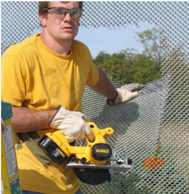
***The 1/2" mesh by 9 GA met a Medium Aggression threat level of M10.9 and outperformed a major competing expanded metal panel product.***
